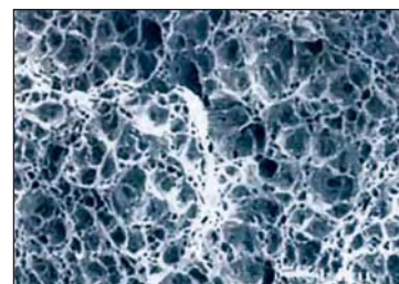
LEFT: Main steam line creep rupture (approx. 10 feet long) at a large fossil utility plant. ABOVE: The SEM photo shows the dimpled fracture/void formation indicative of this type of failure.
