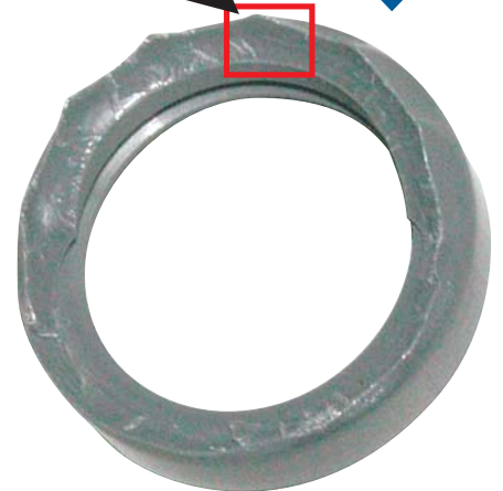
Plastic device fractured by repeated sterilizations
